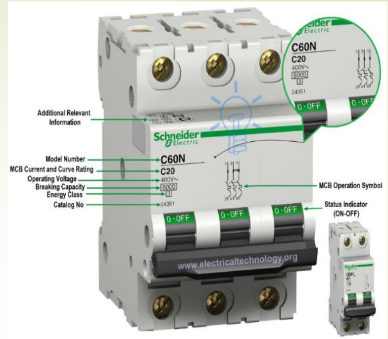
How to Read MCB Nameplate Rating Printed on It
