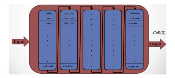
Fig. 5.9 (a): The time interleaving operation for the first clock
