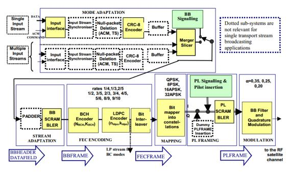
Fig.2.6: DVB-S2 Block Diagram [22]
