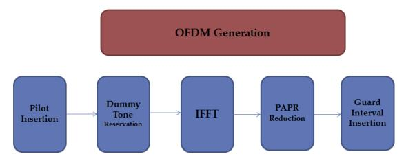
Figure 3.19: OFDM generation Block
