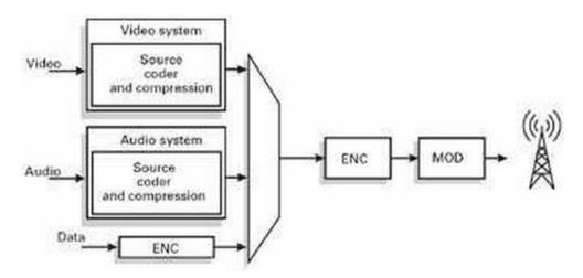
Fig 2.2 ISDB Block Diagram [20]
