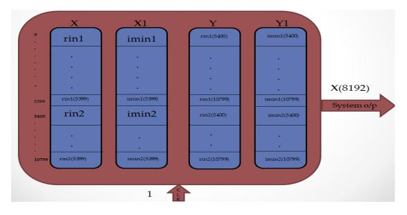
Figure 5.15 (b): The frequency interleaving operation of the second output **5.3.2.3 Combining the cell mapper with the frequency interleaver**
