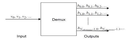
Fig. 3.10: De-multiplexing of bits into sub-streams [29]
