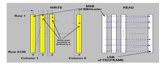
Fig.3.9: Bit interleaving scheme [29] Table 3.2: Column twisting parameter *t*c [2]
