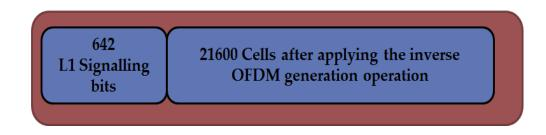
Fig 4.14: The frequency de-interleaver input data stream
