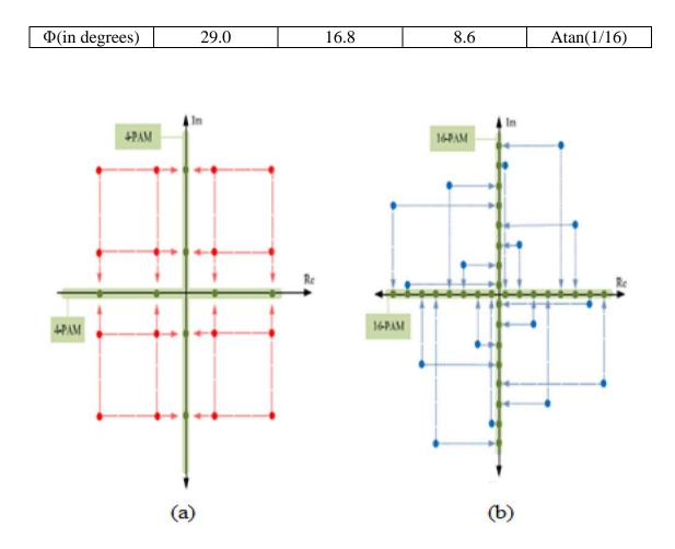
Figure 3.12: a) Classic 16-QAM constellations with projections in axis (2x 4-PAM). b) Rotated 16-QAM constellations with projections in axis (2x16-PAM) [29].
