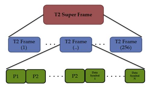
Fig. 3.17: Cell Mapper Frame Structure
