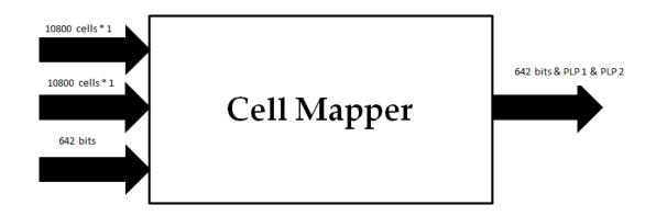
Fig. 4.9: The cell mapper input output dimensions
