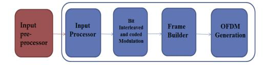
Fig.3.1: High level T2 block diagram
