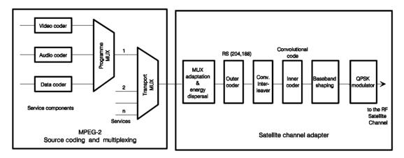
Fig.2.4: DVB-S Block Diagram [22]
