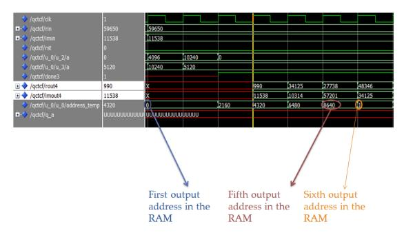
Figure 5.12 (f): The QCT module output sequence
