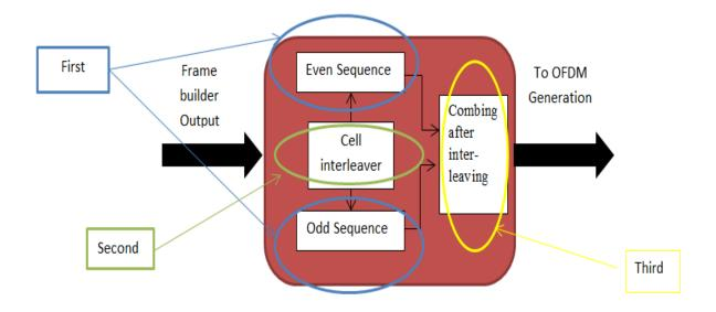
Fig.4.10: Frequency interleaver operation
