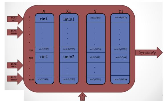
Figure 5.16: The combination of cell mapper with frequency interleaver operations
