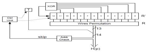
Figure 3.18: Frequency interleaver algorithm for the 16k mode [29] **3.2.4 OFDM generation**
