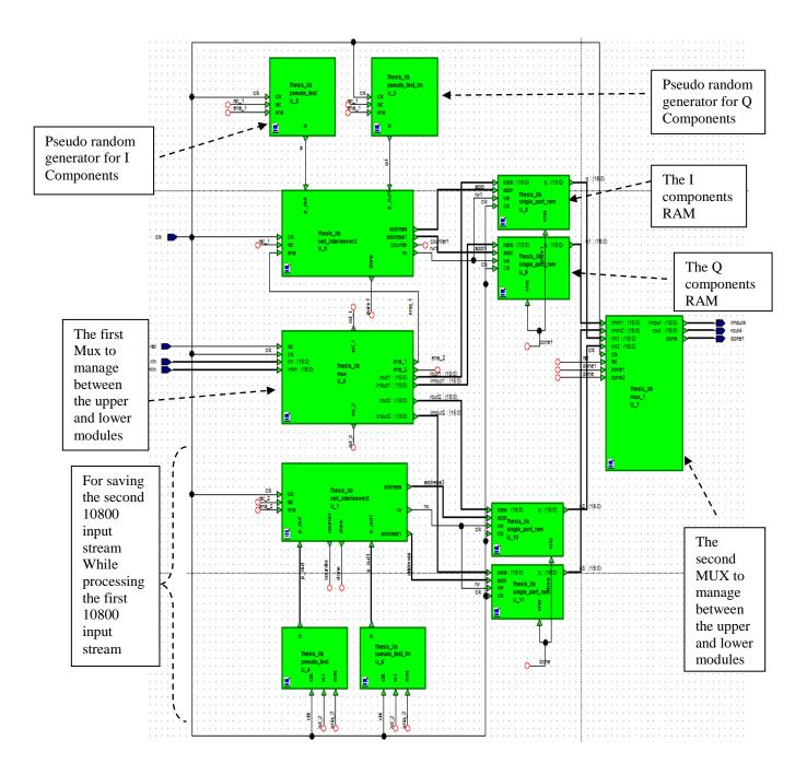
Figure 5.11: The internal QCT Module
