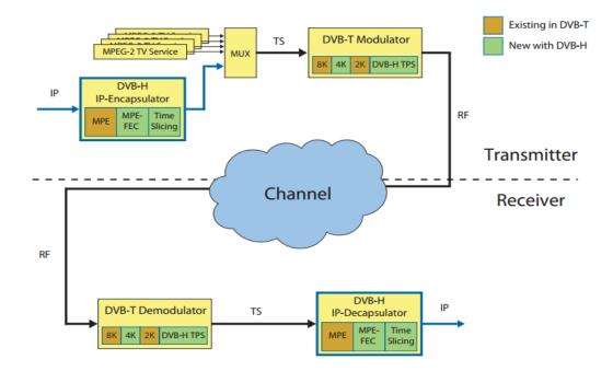
Figure 2.10: Additions brought to the DVB-T system by DVB-H [27]
