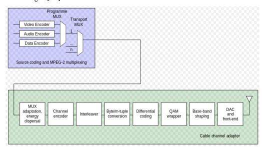
Figure 2.7: DVB-C Block Diagram [25]
