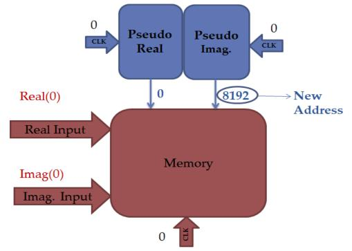
Fig. 5.8 (a): The combined operation for the first clock
