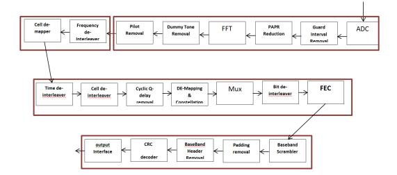
Figure 3.21: DVB-T2 system Receiver
