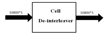
Fig.4.17: Cell de-interleaver input output dimensions
