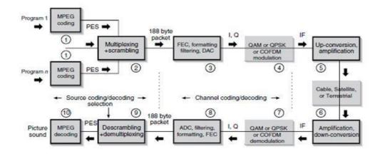
Fig. 2.3: DVB Block Diagram [21]
