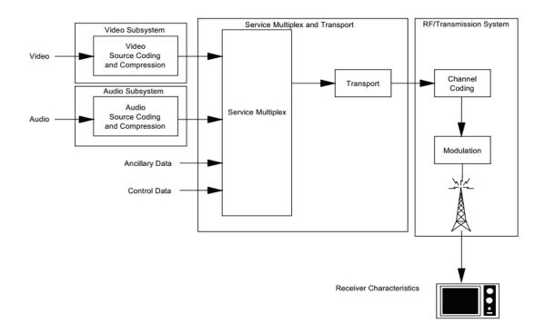
Fig. 2.1: ATSC Block Diagram [19]
