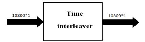
Fig.4.6: Time interleaver input output dimensions
