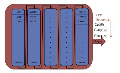
Fig.4.7: Time interleaver operation for 64 QAM
