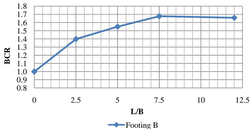
Figure 24: BCR vs.  $L/B$  for footing (B)
