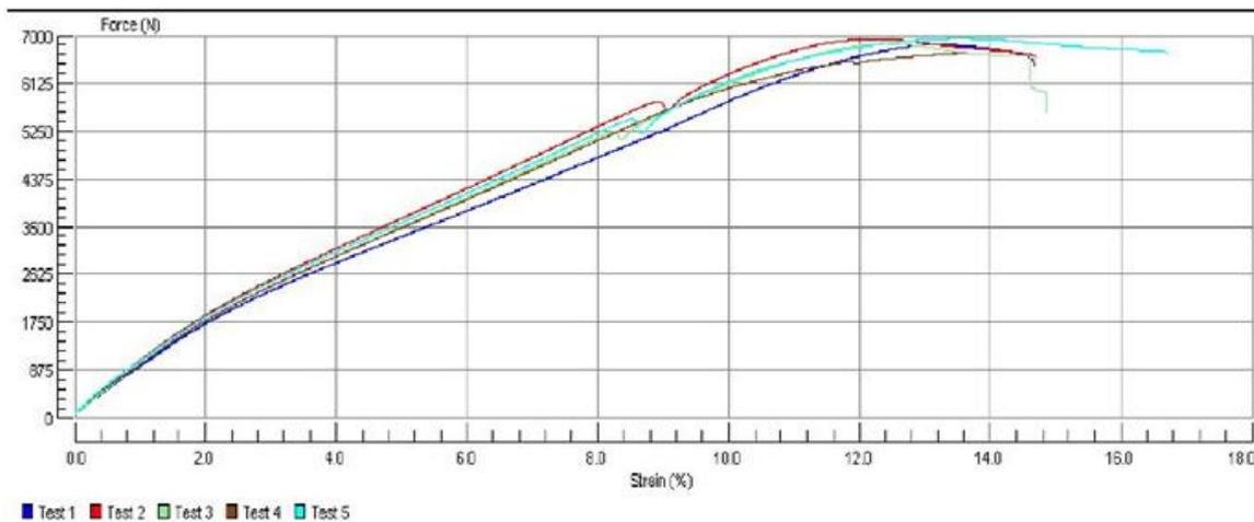
Figure 9: Results of TENAX TT 045 GS uniaxial (Method B)
