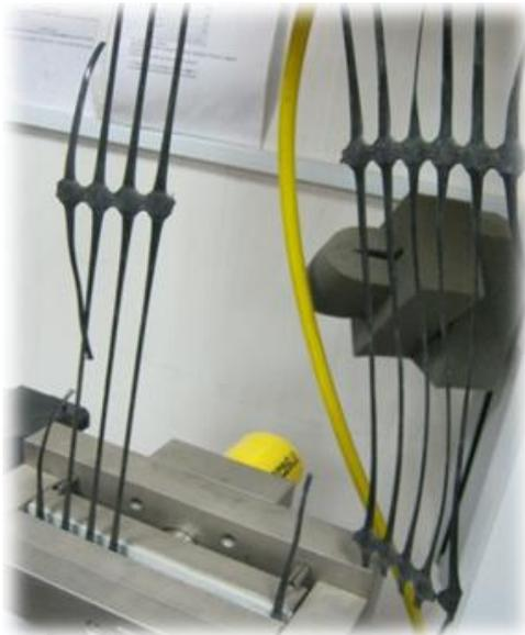
**Figure 6:** Geogrid Junction Rupture
