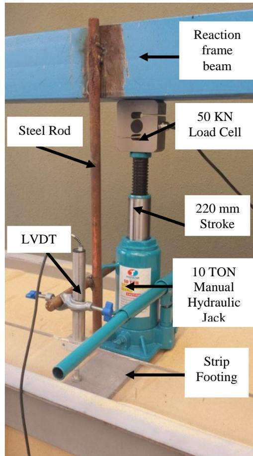
Figure 12: The loading system with measuring instruments
