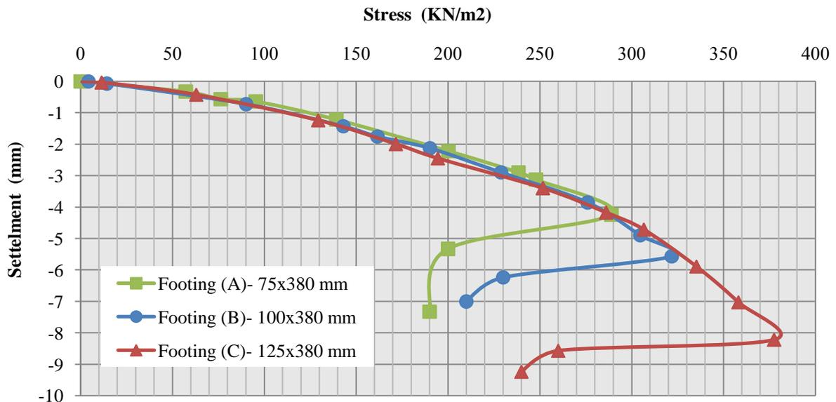
Figure 18: Unreinforced Soil bed Experimental results
