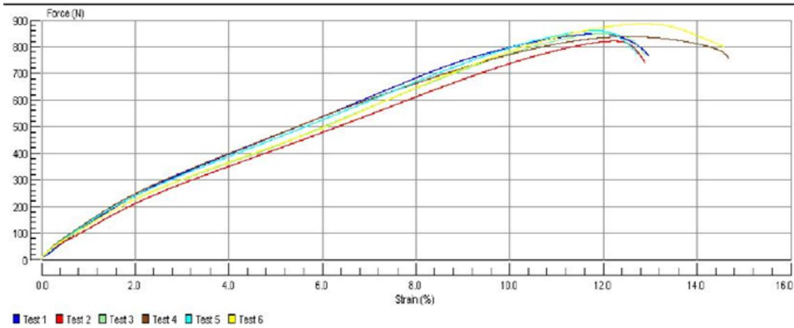
Figure 8: Results of TENAX TT 045 GS uniaxial (Method A)
