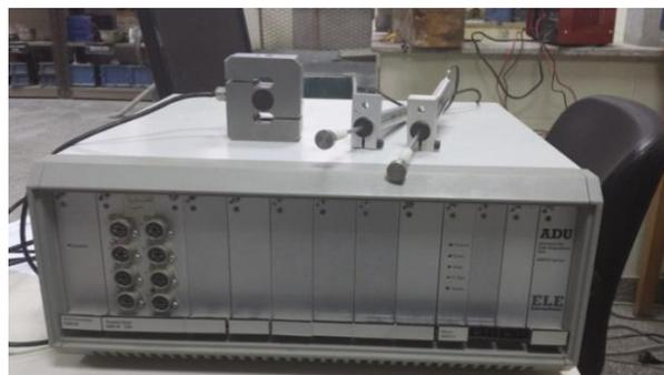
Figure 13: Data acquisition unit
