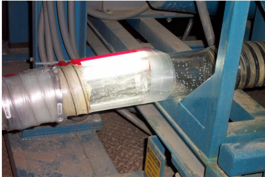
Figure 4.6: Sasobit flowing from distribution box to feeder tube.
