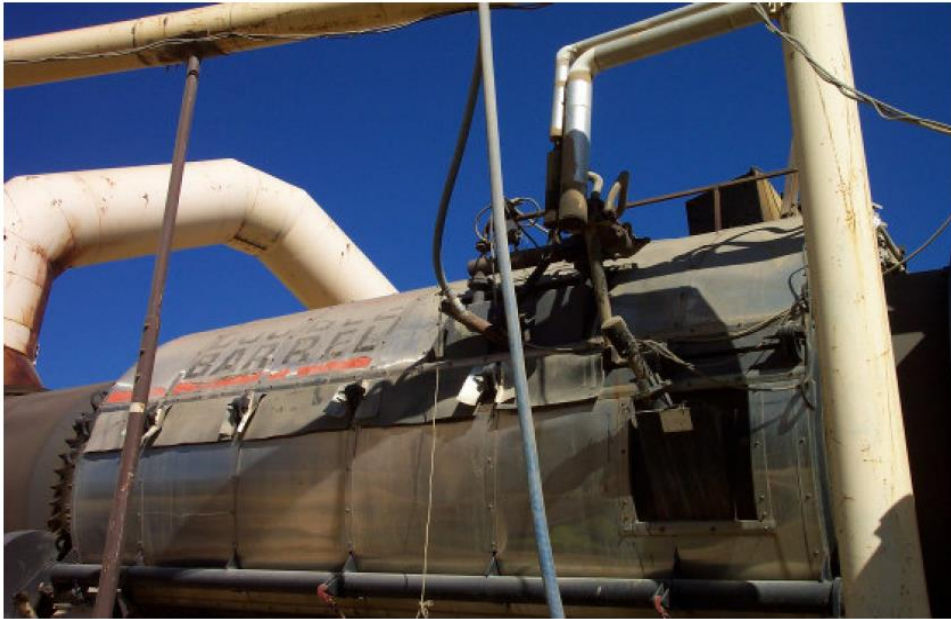
Figure 4.4: Plant retrofitted for Sasobit wax addition.
