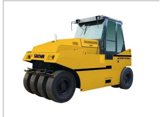
Figure 2.6 Pneumatic Roller Compactor
