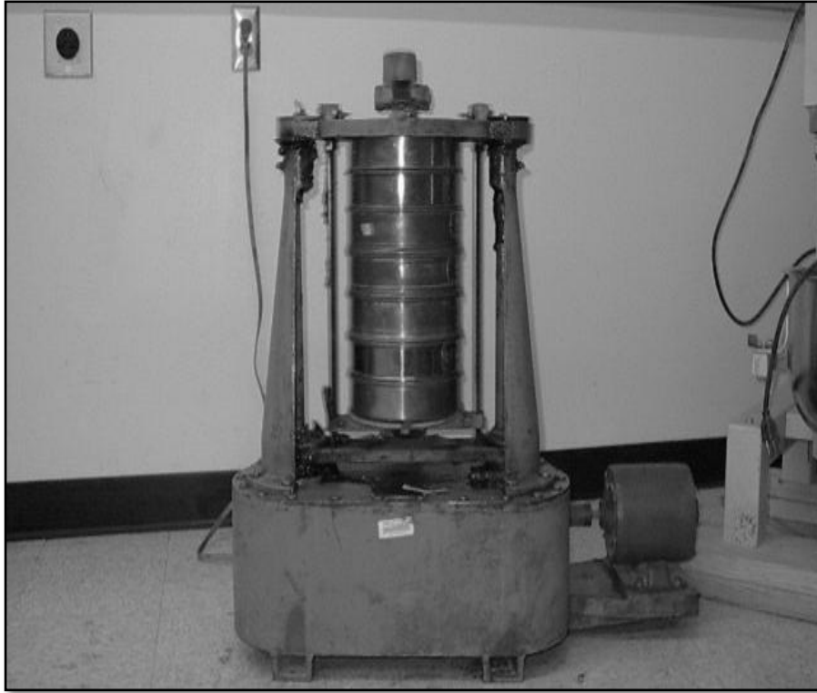
Figure 2.7 The Sieve Shaker with a Stack of Sieves.(instruments,2014)
