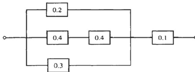
50. The relay network shown in the following figure operates if and only if there is a closed path of relays from left to right. Assume that relays fail independently and that the probability of failure of each relay is as shown. What is the probability that the relay network operates?
