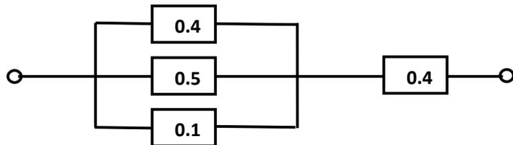
49. The relay network shown in the figure operates if and only if there is a closed path of relays from left to right. Assume that relays fail independently and that the probability of failure of each relay is as shown. What is the probability that the relay network **will not operate**?
