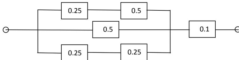
51. Consider the switching network shown in the following figure. It is equally likely that a switch will or will not work. Find the probability that a closed path will exist between terminals a and b.
