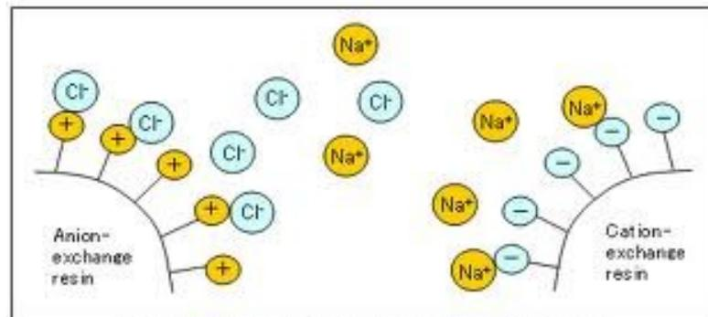
Figure 1. Pattern diagram illustrating ion exchange mode
