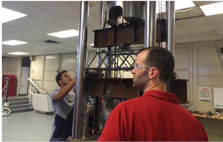
Students taking measurements and checking stresses during the loading test
