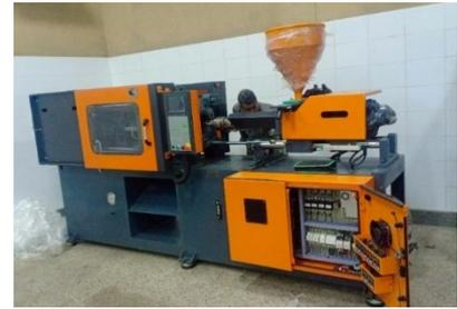
Figure9 Plastic Injection Machine
