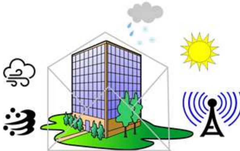
Figure 1 Building envelope separator between the conditioned and unconditioned environments such as air, water, heat, light, and noise.
