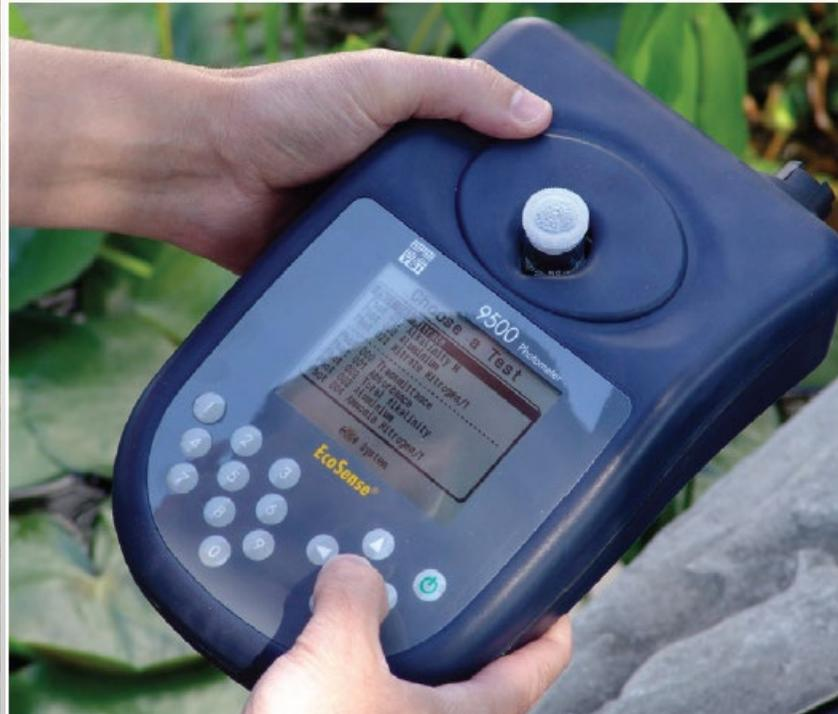
The photometer is suitable for use in both the laboratory and the field.
