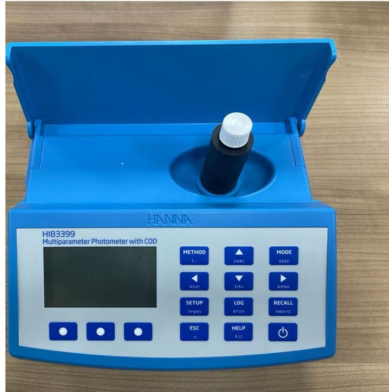
HI83399 benchtop photometer measures 40 different key water and wastewater quality parameters using 73 different methods that allow for multiple ranges and variations in chemistry for specific applications. The Chemical Oxygen Demand (COD) parameter is included for industrial and municipal wastewater treatment.
