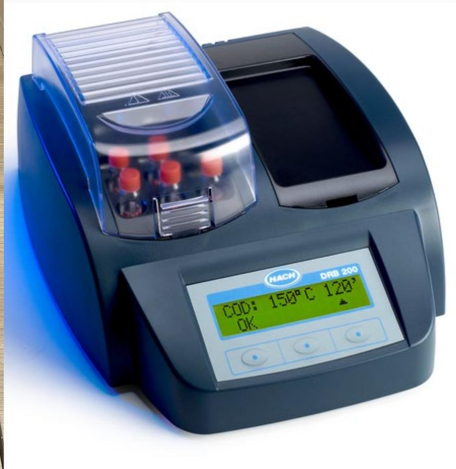
The DRB2000 is used to estimate water pollution levels entering and leaving wastewater treatment and industrial facilities.
