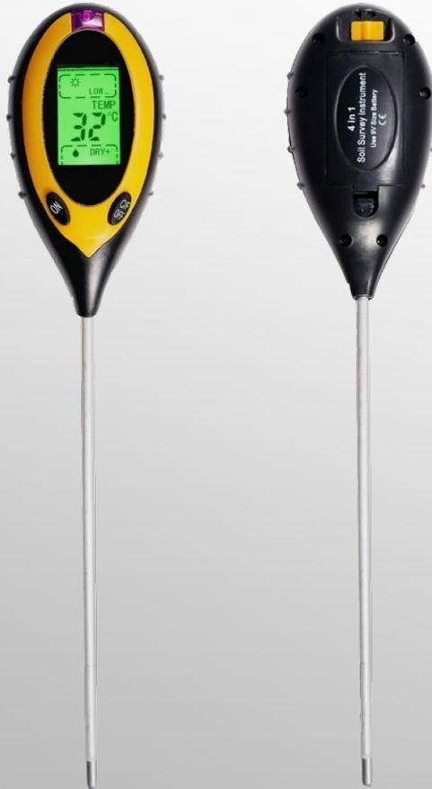
The 4 in 1 soil survey instrument can test moisture of soil, PH value, temperature, and environment sunlight intensity using a probe with a length of 200mm. It can easily display various readings on its oversized LCD, making it easy to read at a glance.
