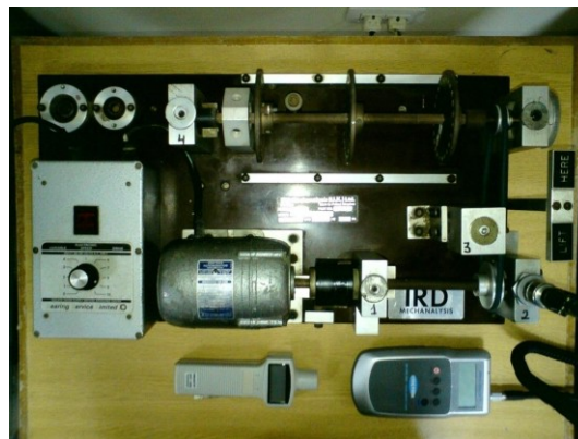
Figure 1.21 Vibration fault kit
