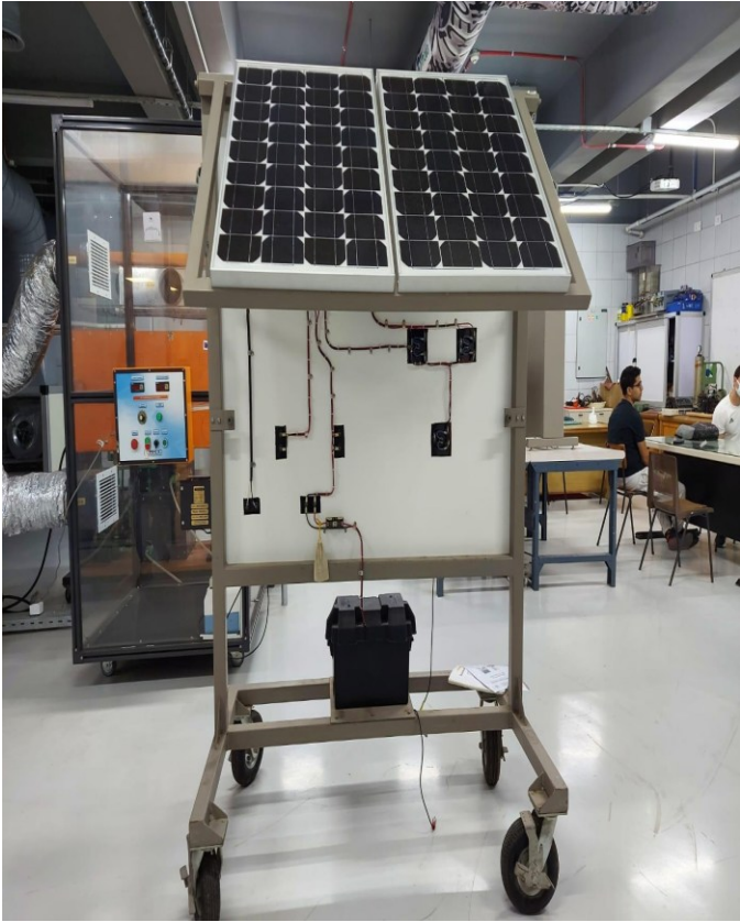
Figure 1.34 Solar Photovoltaic Demonstrator
