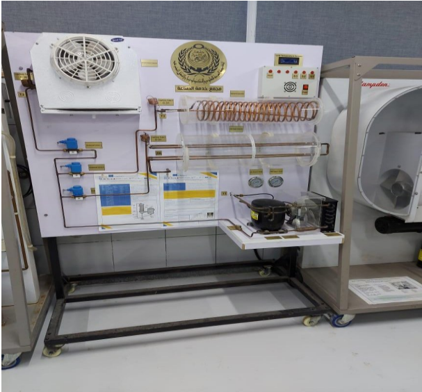
Figure 1.29 Refrigerating cycle trainer
