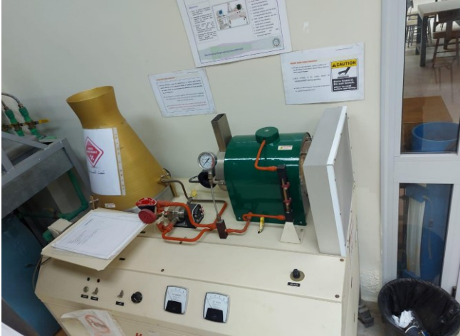
Figure 1.14 Steam power plant
