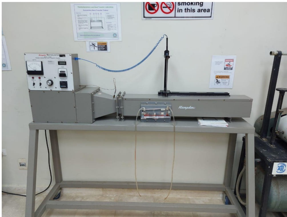
Figure 1.18 Convection heat transfer apparatus
