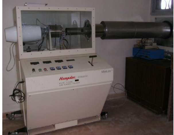
Figure 1.15 Gas Turbine Trainer
