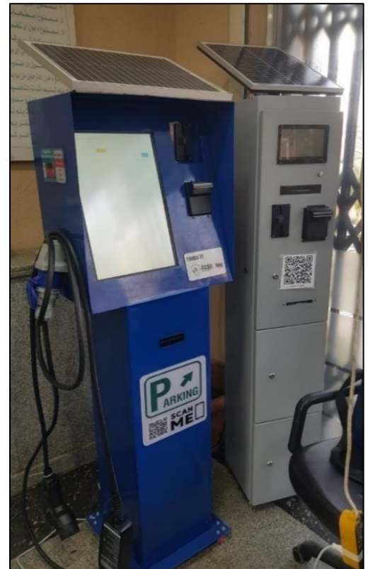
Figure 5. Smart Solar-Powered Parking System
