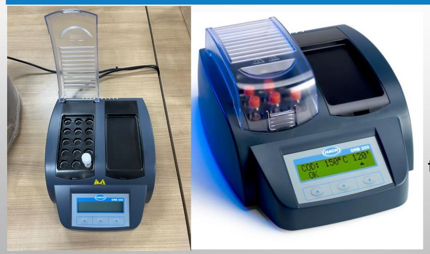
The DRB2000 is used to estimate water pollution levels entering and leaving wastewater treatment and industrial facilities.
