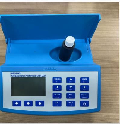
HI83399 benchtop photometer measures 40 different key water and wastewater quality parameters using 73 different methods that allow for multiple ranges and variations in chemistry for specific applications. The Chemical Oxygen Demand (COD) parameter is included for industrial and municipal wastewater treatment.
