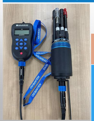
The AP-7000 comes with all of the common water quality testing sensors pre fitted to the probe: pH, ORP, Conductivity, TDS, SSG, Resistivity, Salinity, Dissolved Oxygen, Depth, Temperature.
