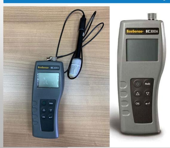
Portable Conductivity, Salinity and Temperature: The EC300A offers convenient conductivity, specific conductance, salinity, total dissolved solids, and temperature with a super-stable, four-electrode conductivity cell for true field applications.
