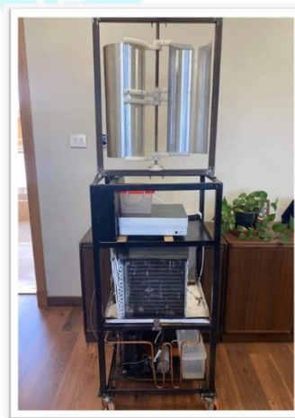
Wind powered atmospheric water generator (AWG) extracts
