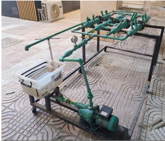
Energy losses in hydraulic piping system
