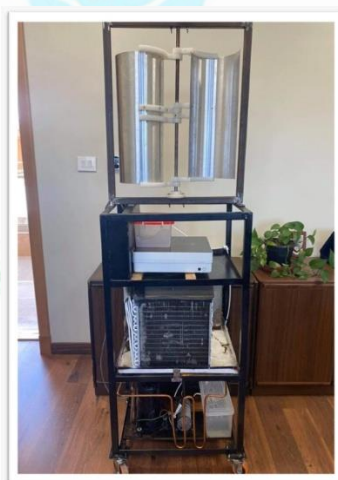
Wind powered atmospheric water generator (AWG) extracts
