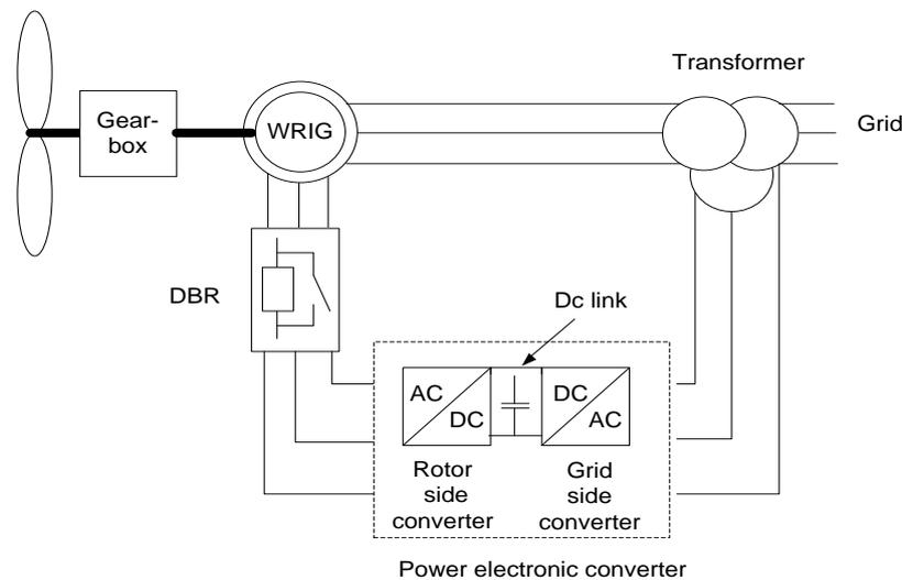
**Fig. 3.9 DFIG with DBR connected to rotor**
