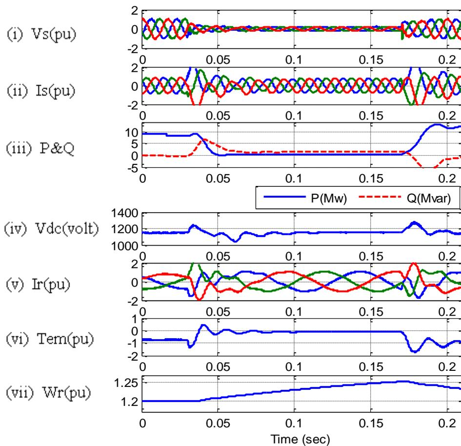
**Fig. 4.3 Symmetrical fault with no protection applied**
