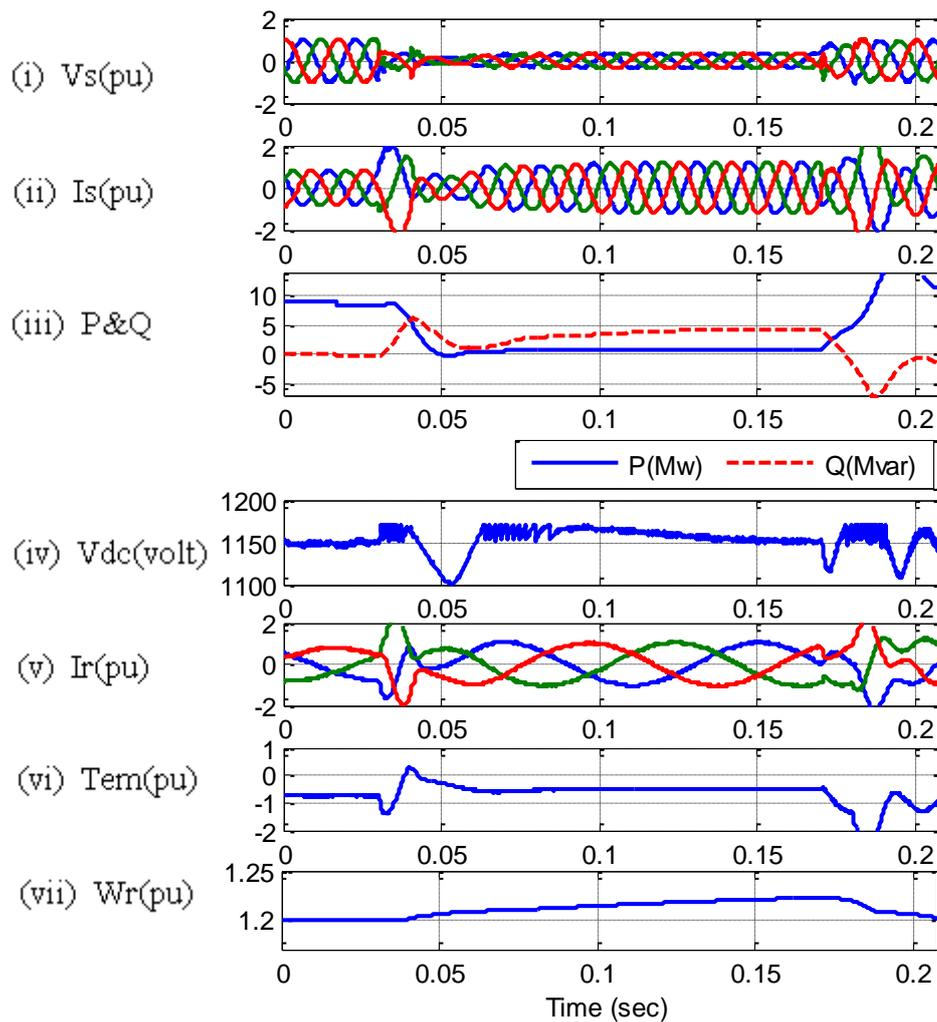
**Fig. 4.22 Symmetrical fault at stator connected DBR (0.02  $\Omega$ )**
