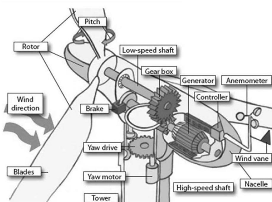
Fig. 2.8 Typical wind turbine system
