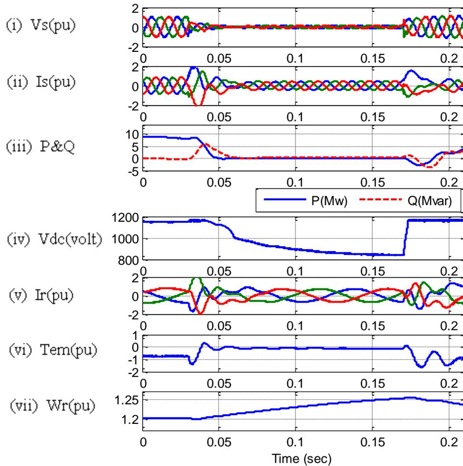
**Fig. 4.16 Symmetrical fault at rotor connected DBR (0.005  $\Omega$ )**
