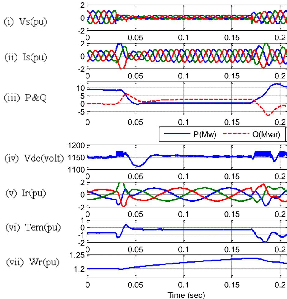
**Fig. 4.21 Symmetrical fault at stator connected DBR (0.01  $\Omega$ )**
