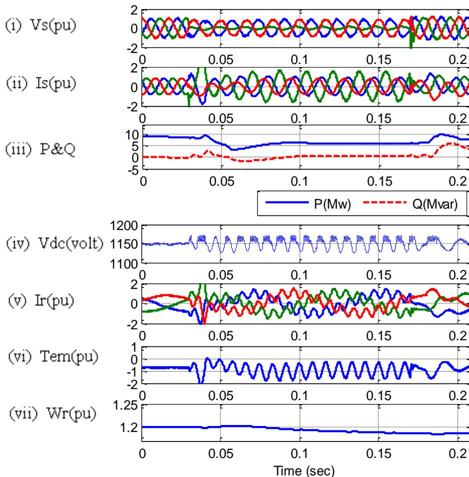
**Fig. 4.19 Asymmetrical fault at stator connected DBR (0.02  $\Omega$ )**
