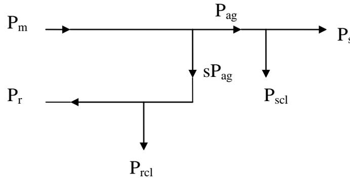
**Fig. 3.3 The power flow diagram of the DFIM in super-synchronous mode**
