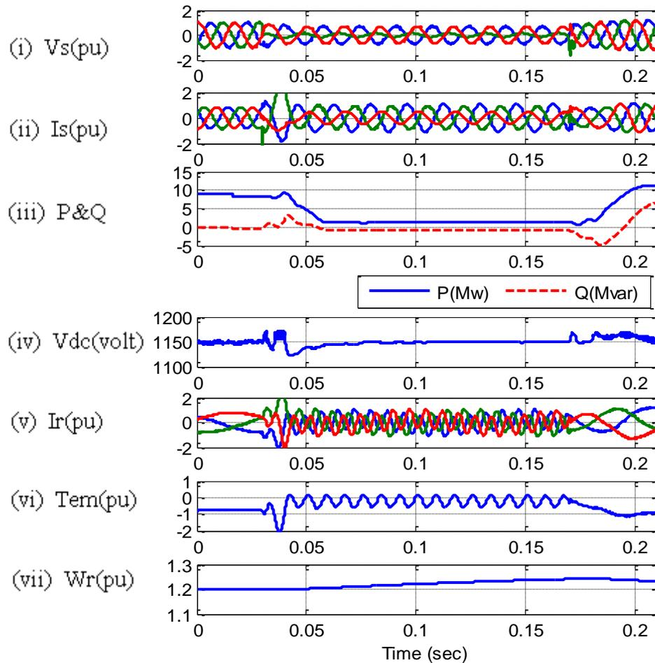
**Fig. 4.7 Asymmetrical fault at CB resistance ( $0.009\ \Omega$ )**
