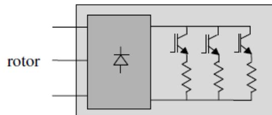
**Fig. 3.8 Active crowbar with a set of various resistors [10]**
