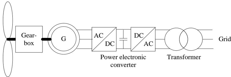
**Fig. 2.12 Variable speed wind turbine**
