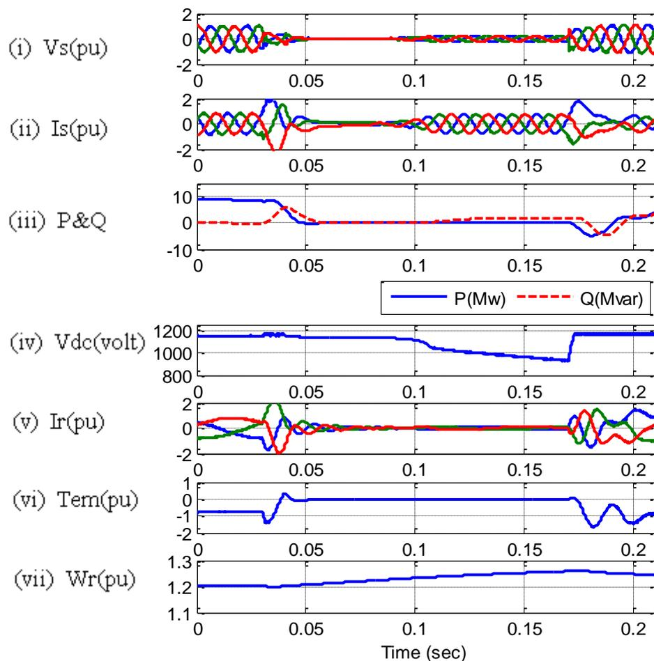
**Fig. 4.11 Symmetrical fault at CB resistance (0.0108  $\Omega$ )**
