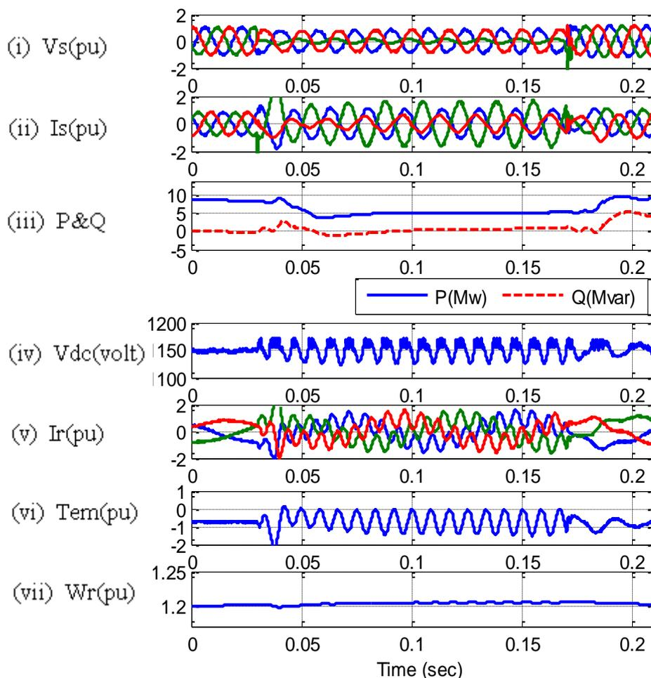
**Fig. 4.18 Asymmetrical fault at stator connected DBR (0.01  $\Omega$ )**
