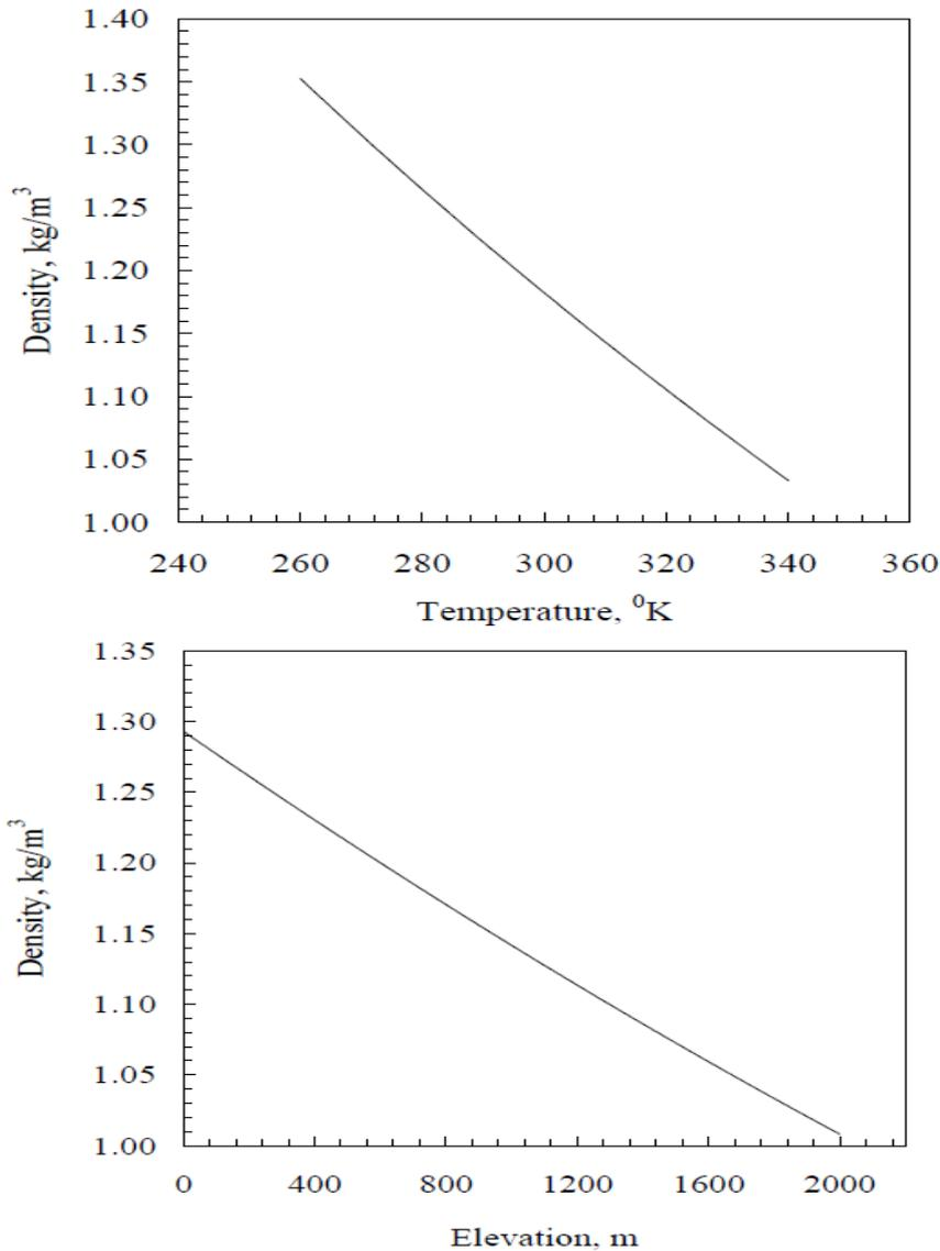
**Fig. 2.5 Effect of elevation and temperature on air density [4]**
