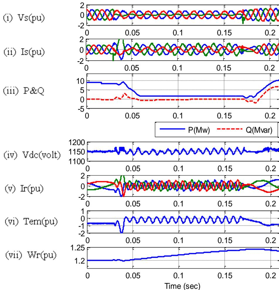
**Fig. 4.14 Asymmetrical fault at rotor connected DBR (0.0125  $\Omega$ )**
