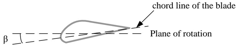
Fig. 2.6 Definition of the pitch angle  $\beta$
