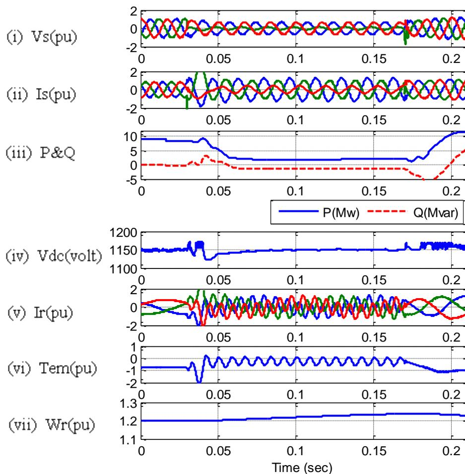
Fig. 4.6 Asymmetrical fault at CB resistance (0.0045  $\Omega$ )
