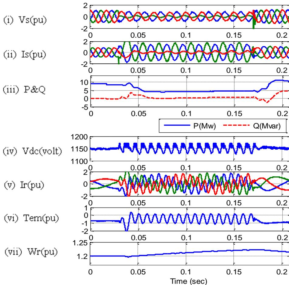
**Fig. 4.4** Asymmetrical fault with only DC chopper technique
