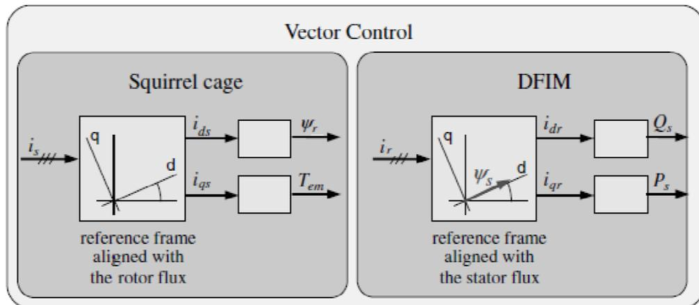
**Fig. 3.5 Comparison between the Vector Control of the squirrel cage machine and the DFIM [10]**
