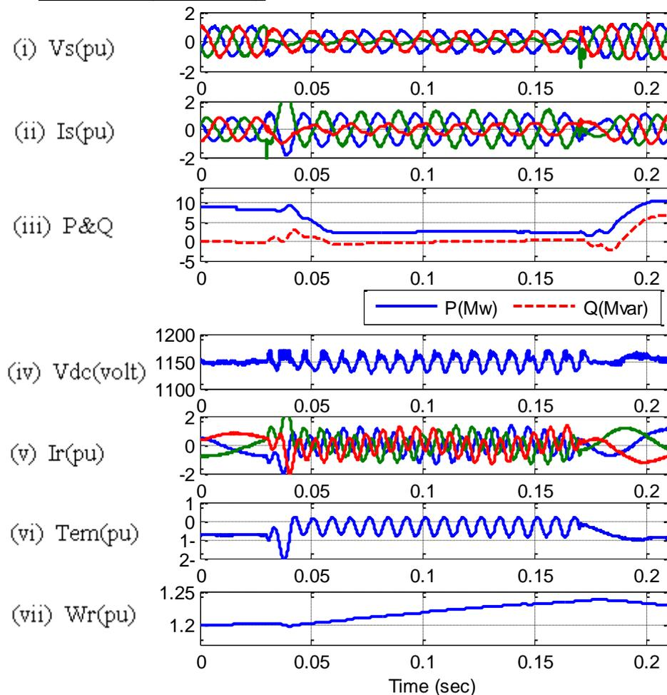
**Fig. 4.13 Asymmetrical fault at rotor connected DBR ( $0.005 \Omega$ )**
