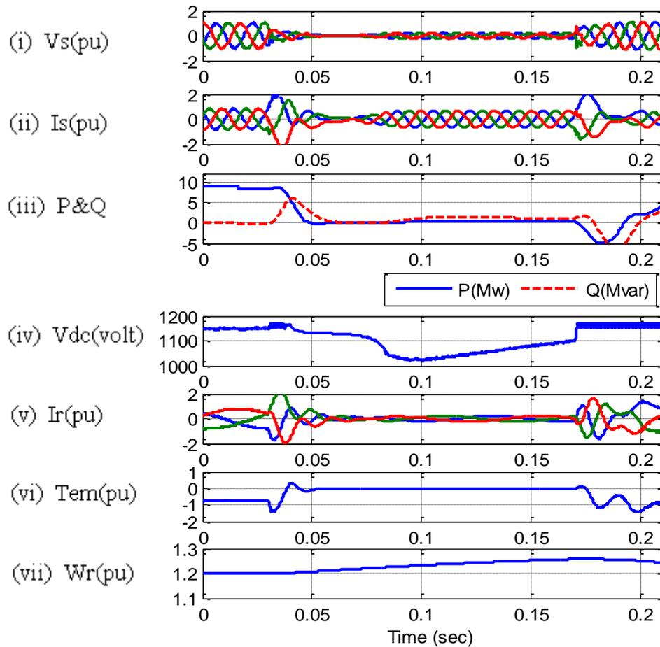
**Fig. 4.9 Symmetrical fault at CB resistance (0.0045 Ω)**
