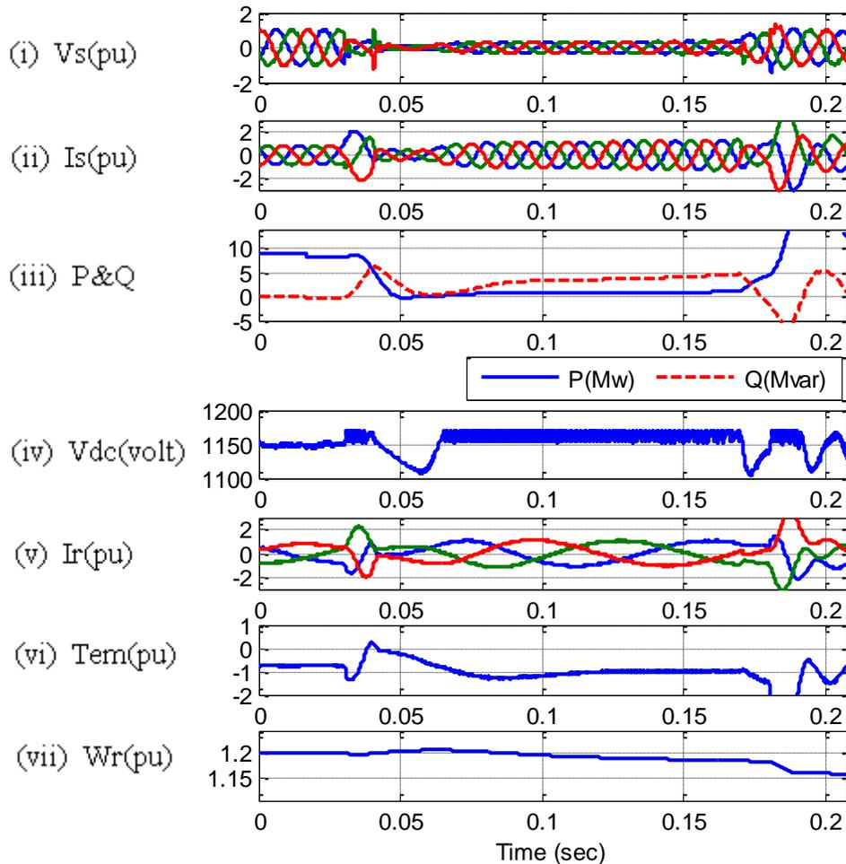
**Fig. 4.23 Symmetrical fault at stator connected DBR (0.05  $\Omega$ )**
