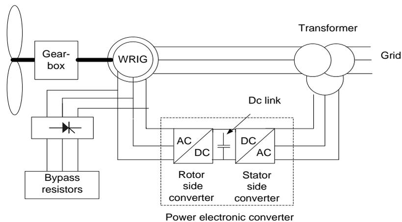
**Fig. 3.11 DFIG with bypass resistors**
