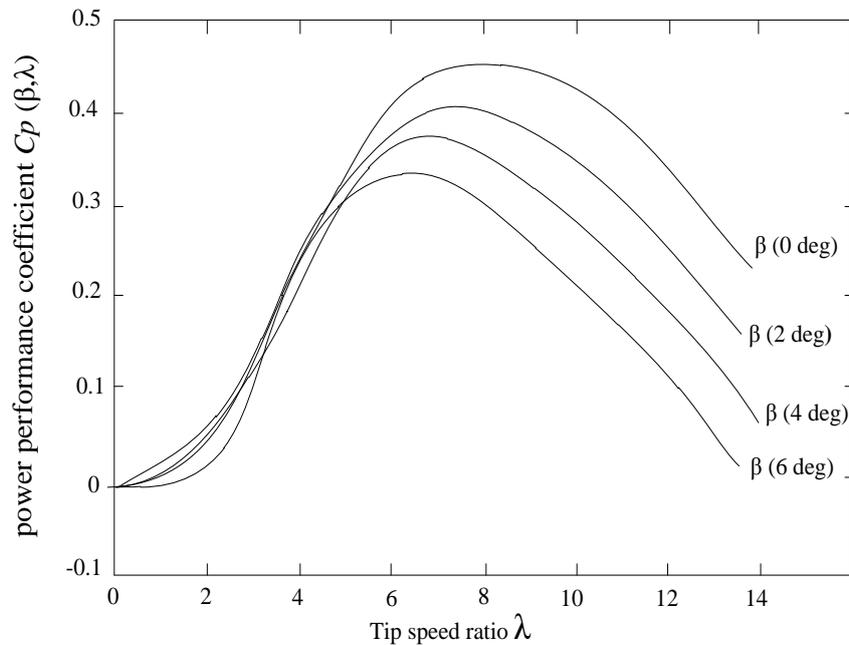
Fig. 2.7 The power coefficient  $C_p$  as a function of the tip speed ratio  $\lambda$  and pitch angle  $\beta$  for a specific blade [7]
