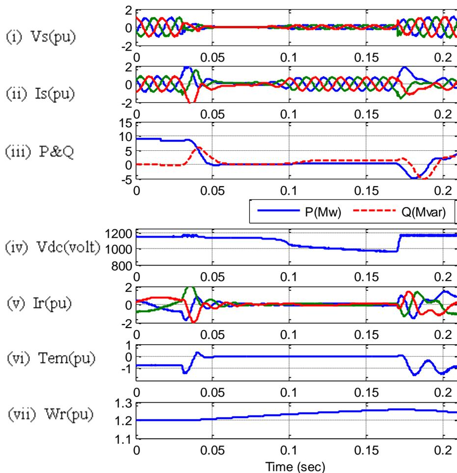
Fig. 4.10 Symmetrical fault at CB Resistance (0.009  $\Omega$ )
