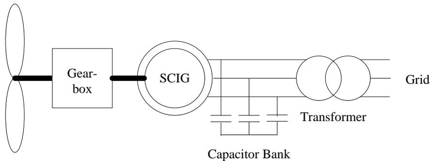
**Fig. 2.11 Fixed speed wind turbine**
