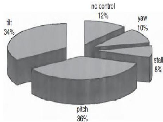
**Fig. 2.10 Speed control methods used in small to medium turbines [9]**
