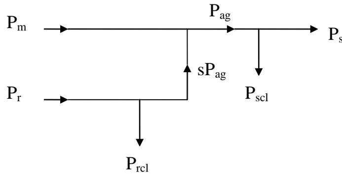
**Fig. 3.4 The power flow diagram of the DFIM in sub-synchronous mode**
