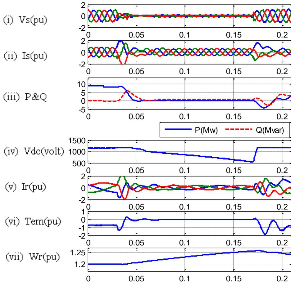
**Fig. 4.17 Symmetrical fault at rotor connected DBR (0.0125  $\Omega$ )**
