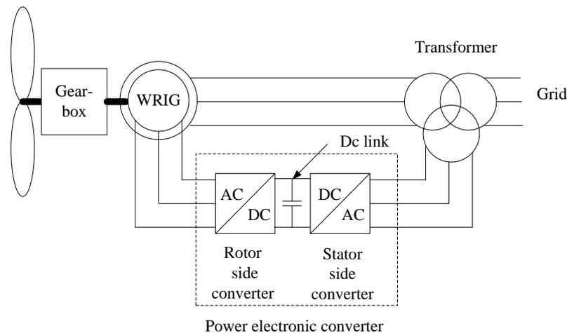
**Fig. 2.13 Variable speed wind turbine**
