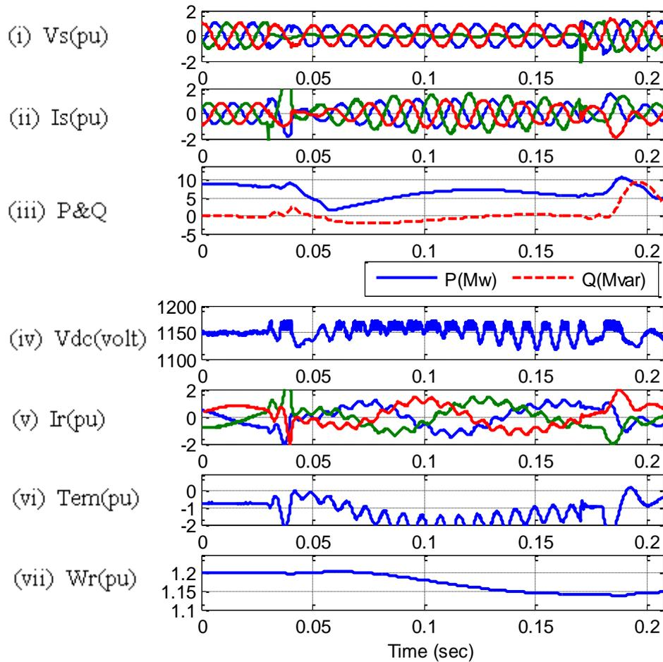
**Fig. 4.20 Asymmetrical fault at stator connected DBR (0.05  $\Omega$ )**
