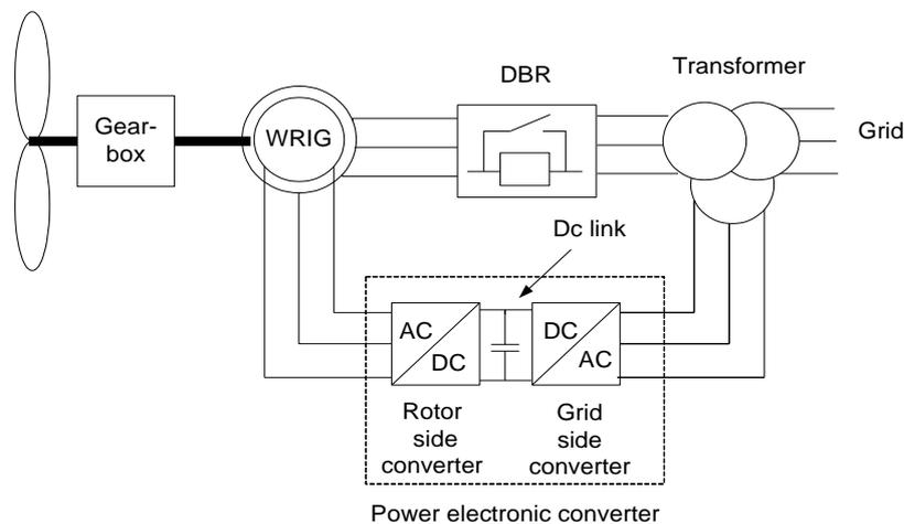
**Fig. 3.10 DFIG with DBR connected to stator**
