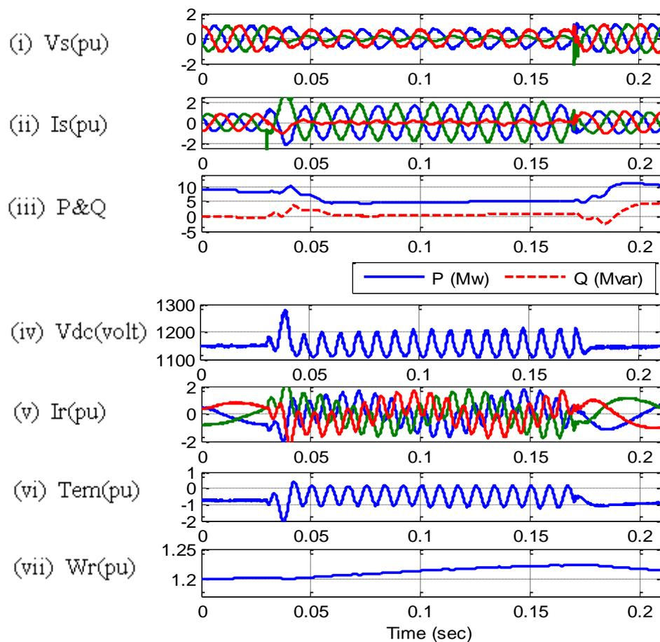
**Fig. 4.2 Asymmetrical fault with no protection applied**
