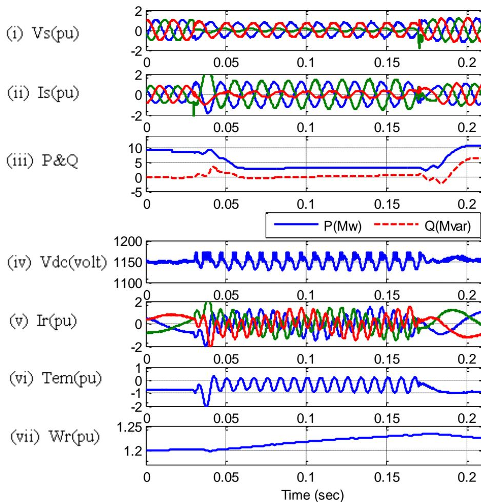
Fig. 4.12 Asymmetrical fault at rotor connected DBR (0.0025  $\Omega$ )
