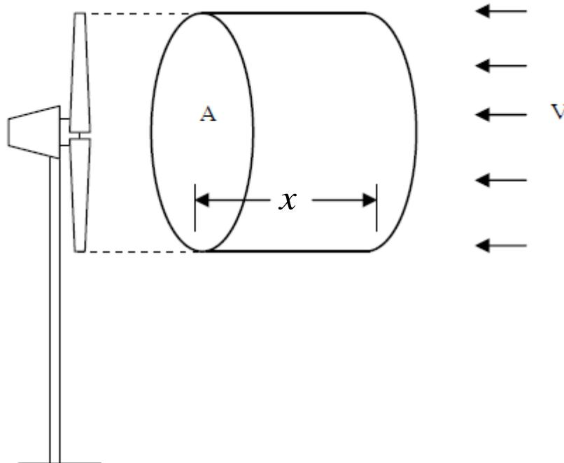
Fig. 2.4 An air mass moving toward wind turbine [4]
