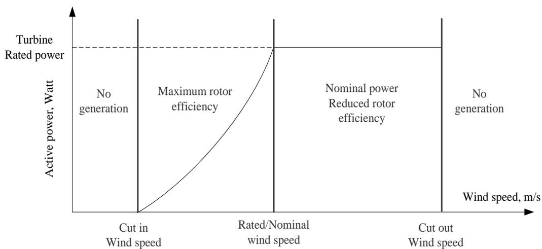
**Fig. 2.9 A typicality power curve of a wind turbine [7]**
