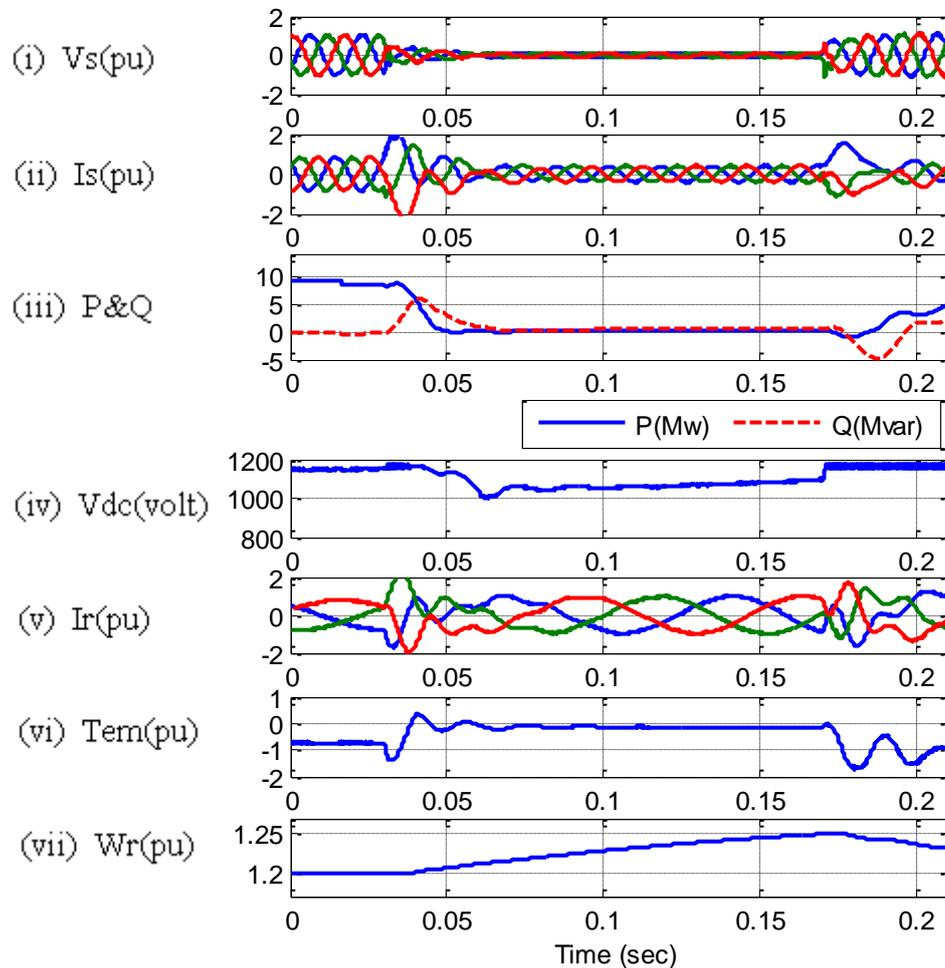
**Fig. 4.15 Symmetrical fault at rotor connected DBR (0.0025  $\Omega$ )**
