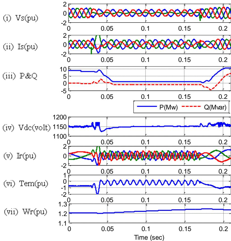
**Fig. 4.8 Asymmetrical fault at CB resistance (0.0108  $\Omega$ )**
