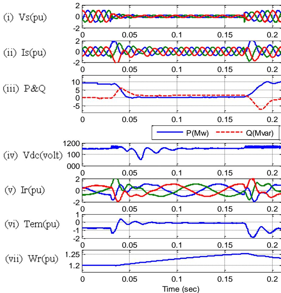
**Fig. 4.5 Symmetrical fault with only DC chopper technique applied**
