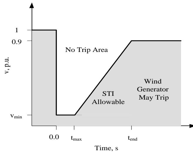
**Fig. 2.14** Fault ride through requirement of wind farms
