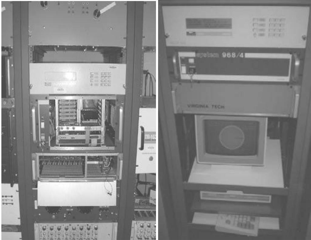
**Fig 3.1** First prototype PMU built at Virginia Tech
