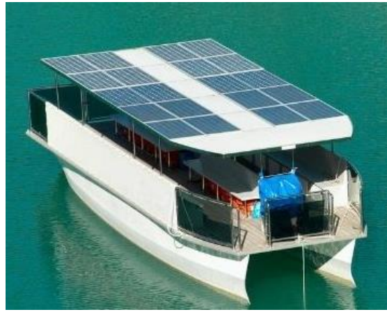
PV-equipped electric river vehicle
