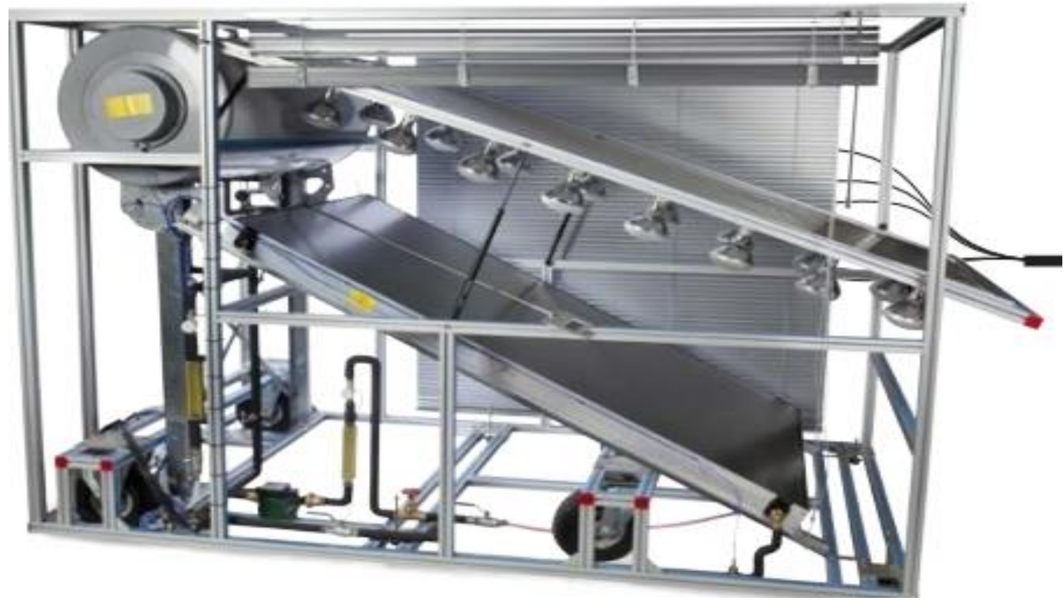
Solar Heater system with sun simulator capacity 300l with digital interface
